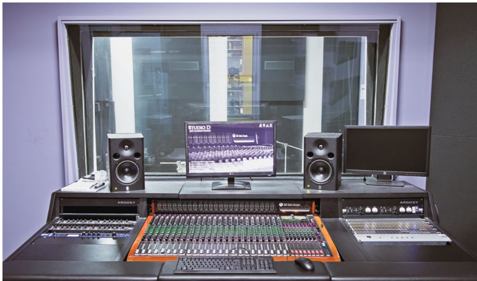
The all-analogue Toft ATB24 recording console, with its clearly delineated functions and signal paths, is the first step for all students training in the craft of recording.
